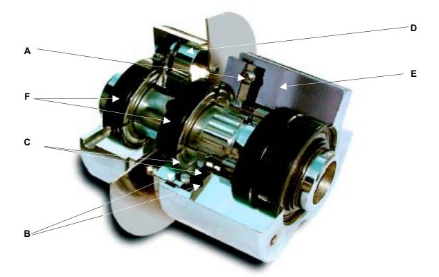
The drive is transmitted through balls 'A' held in detents 'B' in opposing plates 'C' by adjustable air pressure acting on a large annular piston or a number of small pistons depending on the torque required.
